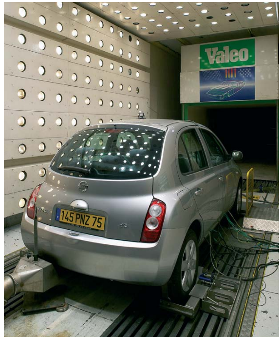
Cool-down testing with sun lamps
