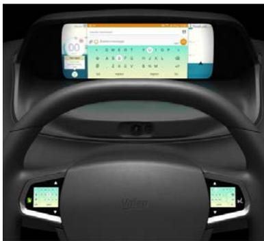
**Whenever Valeo Mobius™ 2 detects favorable conditions for autonomous driving**, for example when the car is in a city traffic jam or on the highway, **it suggests that the driver switch to hands-off mode** by pressing the automatic pilot button located on the steering wheel. Similarly, the system emits a visual and audio alert as soon as it anticipates the need for the driver to resume control.
