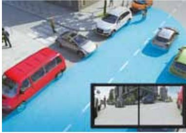
The driver may also select other views on the screen: for example, a wide-angle view of the area behind the vehicle is particularly useful when parking. Similarly, viewing the area in front of the vehicle is important at a blind junction or parking slot exit. The front camera image shows impending cross traffic which is particularly helpful when the driver's view is obstructed.
