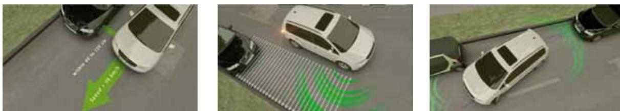
The new version for parallel parking needs only 40 cm of clearance at either end of the vehicle to be able to park, a reduction of 43% compared to the first generation, made possible by a more sophisticated geometric calculation. In addition, steering assistance continues to help the driver until the vehicle is parked, however many manoeuvres may be necessary for a short parking slot.
