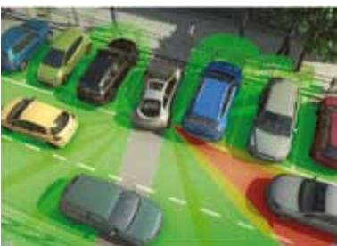
The Blind Spot Monitoring system ensures safe lane changes. Thanks to a radar sensor on either side of the rear of the car it detects any vehicle next to and behind it. The blind spot radar can establish the precise position of all obstacles in the adjacent lane. This information is then analyzed by an algorithmic program to determine the type of obstacle, its relative speed and direction.
