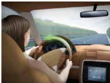
The camera-based LaneGuide™ system, alerts the driver if the vehicle unintentionally leaves the lane and assists by subtly pulling the car back into the lane. The system uses a camera placed behind the windscreen, which tracks the road up to 30 meters ahead of the vehicle. These images are processed by an application monitoring the road markings of the lane in which the car is driving, and can calculate whether the vehicle will stay to its lane on the current trajectory.
