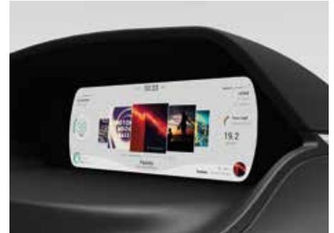
With the Valeo Mobi/us concept, motorists can use smartphone or tablet apps while keeping their hands on the steering wheel and their eyes on the road. Valeo Mobi/us includes a system that detects the presence of hands on the steering wheel and uses a camera to observe the driver.
