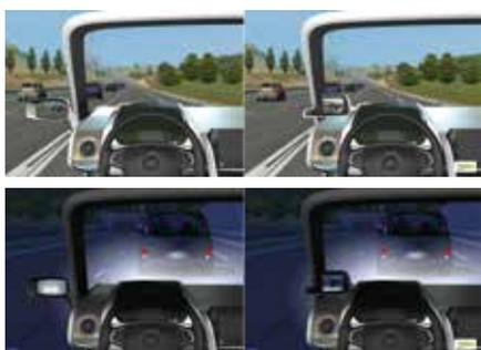
As part of this commitment, Valeo teams have developed Sightstream, a new system that replaces conventional interior and exterior rearview mirrors with cameras. In other words, what used to be seen outside the car is now seen on the inside. This considerably improves vehicle aerodynamics and reduces drag, thereby saving fuel and lowering CO<sub>2</sub> emissions by 1.3 grams per kilometer.
