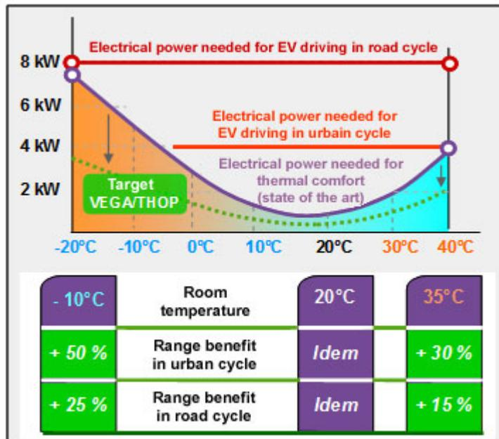
(\*) : VEGA/THOP: (long-range electric vehicle/system for the optimized thermal control of the cabin and the powertrain).
