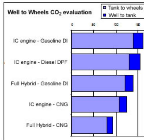
Engines designed to run on petrol can easily be adapted to CNG, but the compression ratio should be increased by about 30% in order to benefit from the increased efficiency. Natural gas is also well suited to turbocharged engines and hybrid powertrains.
