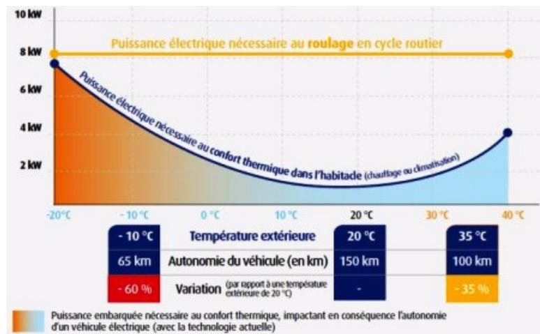
At high ambient temperatures, the air conditioning can consume as much as one half of the power needed to propel the vehicle. In addition, it is becoming increasingly beneficial to drive the compressor using a dedicated motor, rather than the vehicle's drive motor in order to optimize comfort, power consumption and range. In this case, the compressor no longer needs to be located in the engine compartment and can be moved closer to the cabin.
