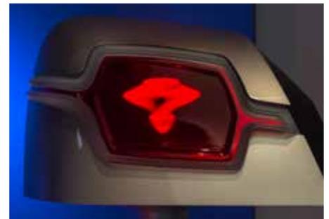
Kinetic rear lights can communicate with the surrounding environment by displaying pictograms or personalized messages. A car in automated driving mode equipped with a Kinetic system can therefore inform the vehicle behind it whenever its sensors detect a hazardous situation.
