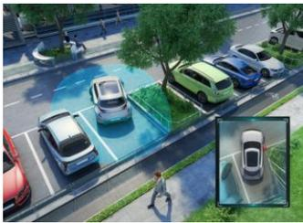
The intuitive and ergonomic [360Vue® 3D](#) system is designed to help drivers maneuver their vehicles with greater accuracy. It works by giving the driver a bird's eye view of the vehicle on the dashboard screen. The 3D, 360-degree image it provides of the surrounding environment ensures full visibility right around the vehicle.
