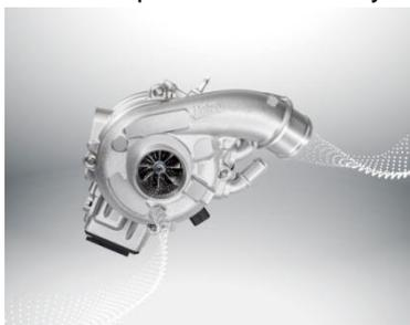
Valeo has developed an electric supercharger that can instantly deliver additional torque to engines at low revolutions. While a turbocharger requires 1.5 to 2 seconds to activate, Valeo's 48V e-supercharger only takes 220 milliseconds, making it 6.8-times faster. The solution can be incorporated into gasoline, diesel and hybrid engines and also adapts to 12V and 48V electric systems.
