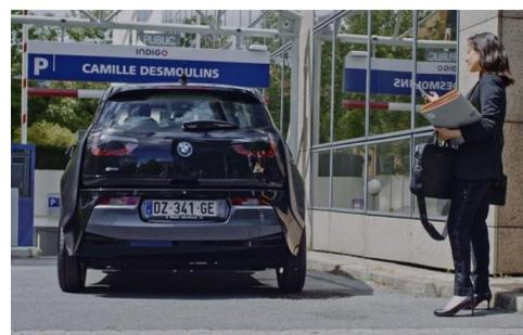
The vehicle drives itself inside the car park by combining the power of automatic parking technologies (**Valeo Park4U®**), Valeo onboard telematics and secure key systems (Valeo InBlue®) with Cisco Parking Controller technologies, which equip car parks with Wi-Fi, video sensors and artificial intelligence-based solutions.
