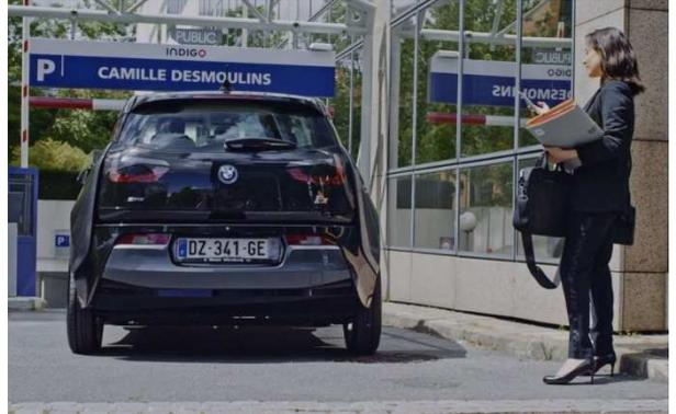
The vehicle drives itself inside the car park by combining the power of automated parking technologies (Valeo Park4U<sup>®</sup>), Valeo onboard telematics and secure key systems (Valeo InBlue<sup>®</sup>) with Cisco Parking Controller technologies, which equip car parks with Wi-Fi, video sensors and artificial intelligence-based solutions.
