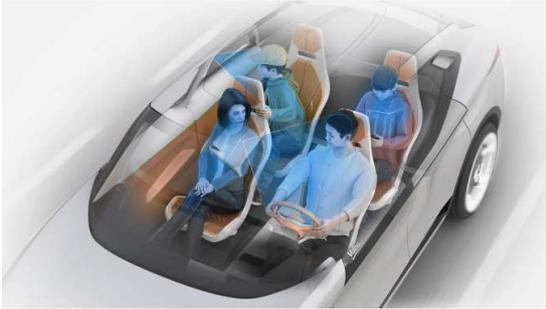
At CES 2018, Valeo is showcasing a solution that detects whether the car is occupied when the engine is off. Sensors in the vehicle cabin identify the number, location and morphology of people present. A vehicle fitted with this Valeo technology will trigger a sound and light alarm, and send a message to the user's smartphone, to ensure that no one is left behind in a stationary car.
